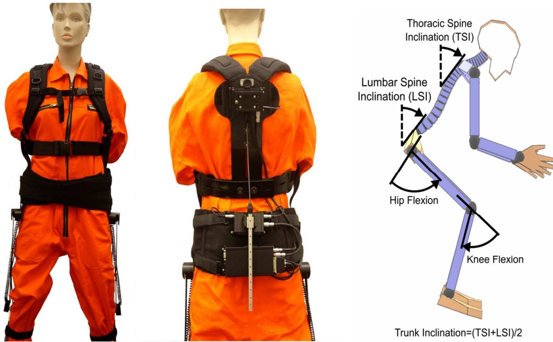
Figure 2: Front and back view of the CUELA measuring system and stick figure to demonstrate the outcome parameters for gait (Note: the direction of the arrows shows the positive direction of the outcome parameter)
