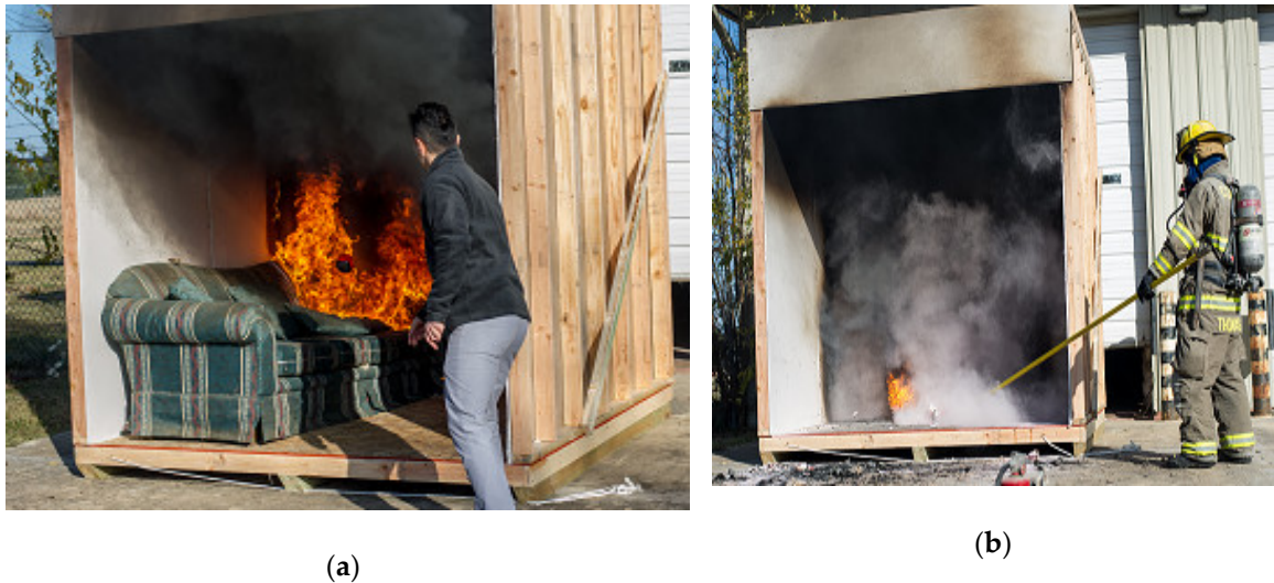
Figure 3. (a) 'Class A' fire in the demonstration cell for the case study; (b) 'Class B' fire in the demonstration cell for the controlled experiments.
